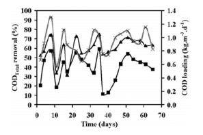
Fig. 5 the COD removal efficiency of two kinds of ASBR and organic loading rate. (Sarti et al., 2007)
