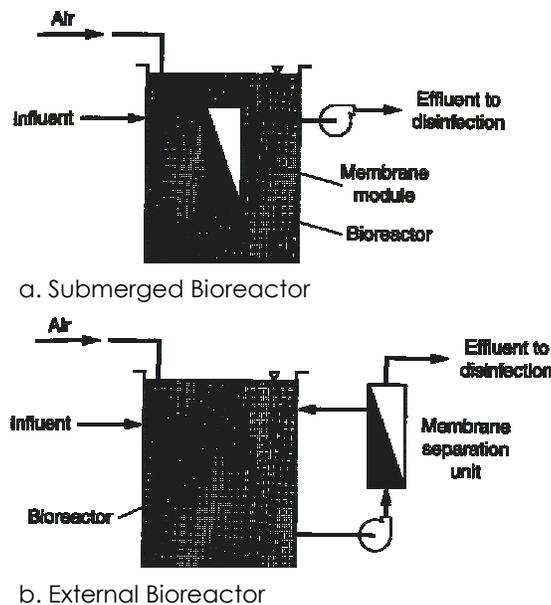
**Figure 4:** Membrane Bioreactors (Metcalf & Eddy, 2003)
