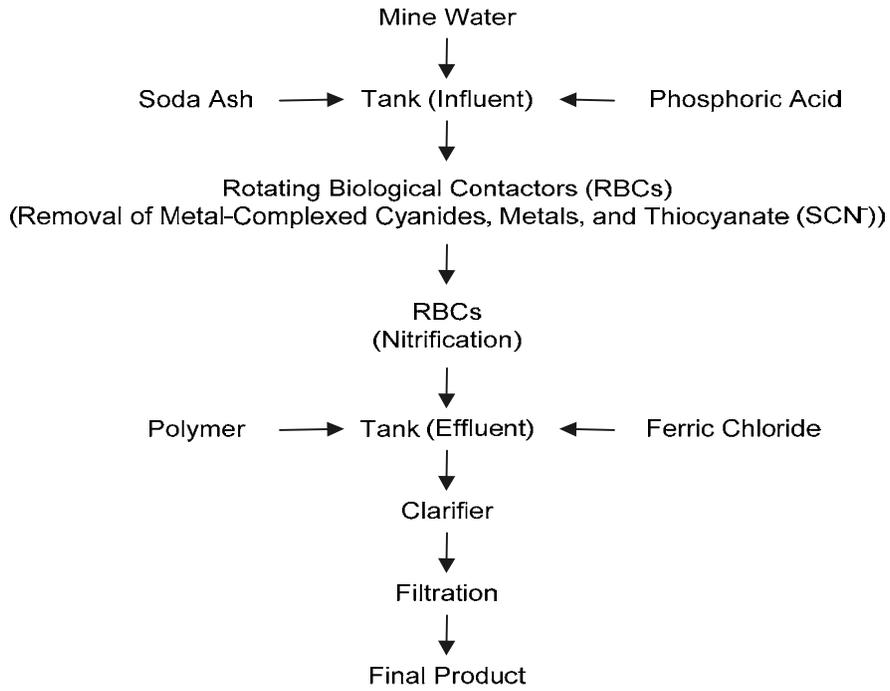
Fig. 3 Mechanisms of Homestake's Aerobic Biological Treatment Process (Akcil 2003)
