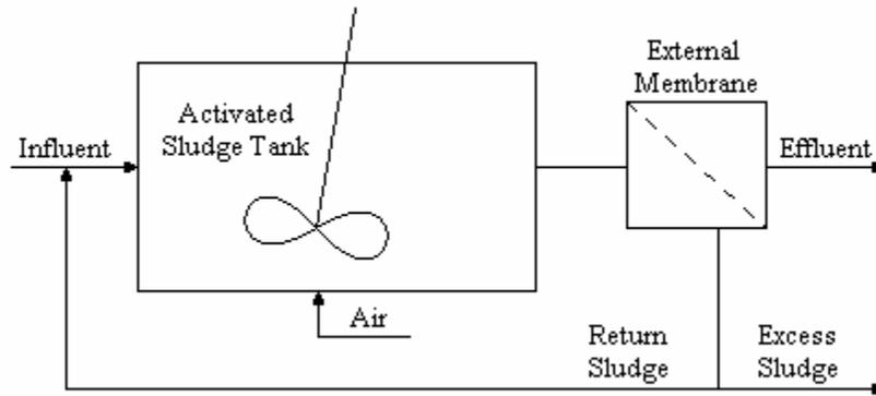
**Figure 14-4.** Membrane-coupled aerobic bioreactor with an external membrane. (Modified from Gnder, 2001.)
