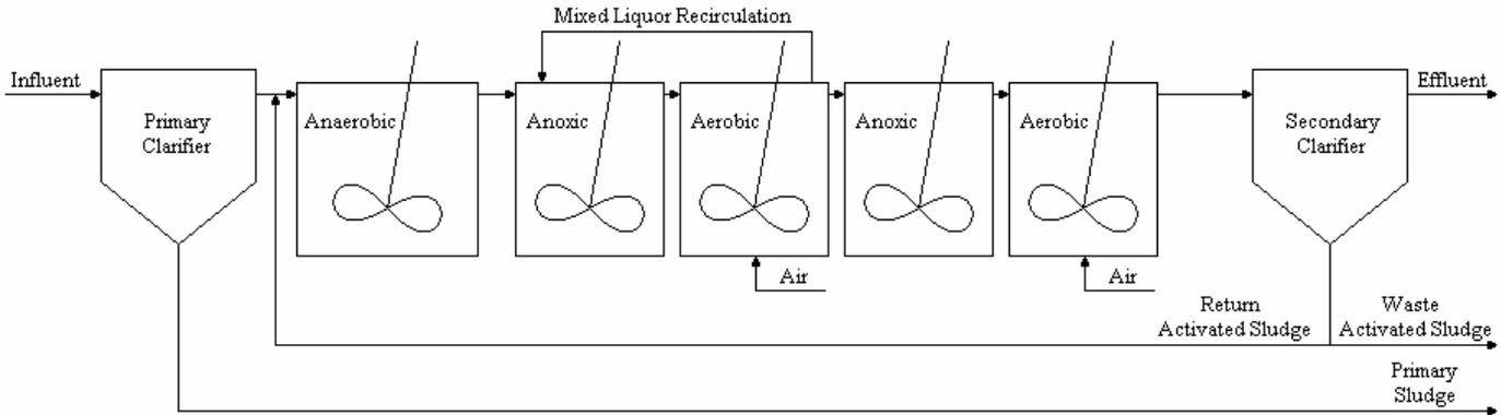
**Figure 14-3.** Activated sludge process with nitrification-denitrification and biological phosphorus removal. (Modified from Winkler, 1981.)
