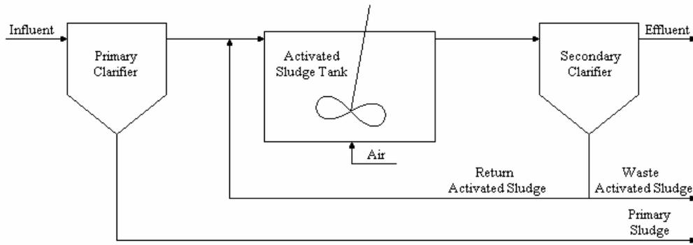
**Figure 14-1.** Traditional activated sludge process. (Modified from Gnder, 2001, and U.S. EPA, 1977.)
