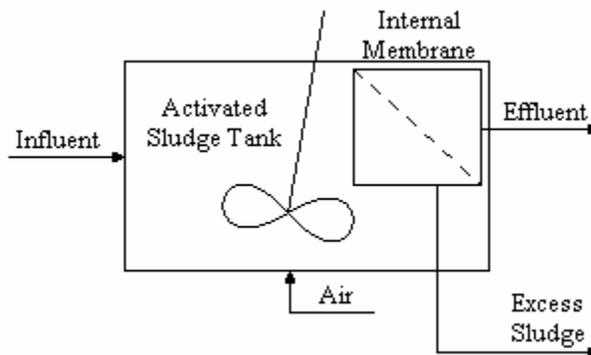
**Figure 14-5.** Membrane-coupled aerobic bioreactor with an internal membrane. (Modified from Gnder, 2001.)
