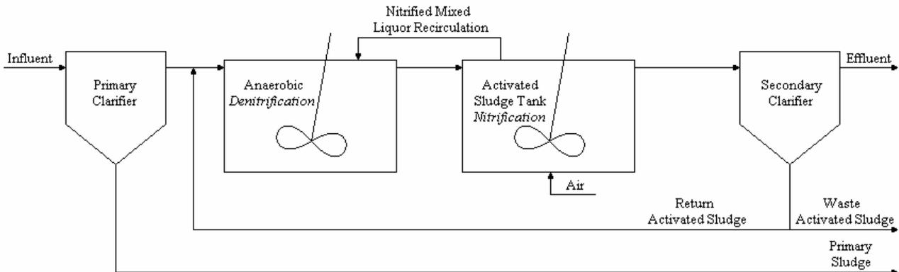
**Figure 14-2.** Activated sludge process with nitrification-denitrification. (Modified from Winkler, 1981.)
