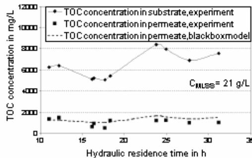
**Figure 14-7.** Comparison of the black box MBR model with experimental data. (From Gehlert and Hapke, 2002.)
