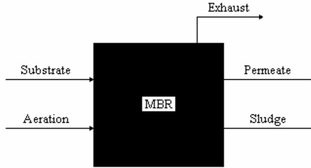
**Figure 14-6.** Black box model of MBR. (Modified from Gehlert and Hapke, 2002.)
