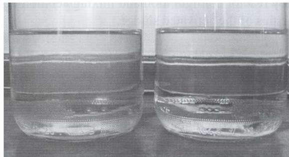
**Figure 14-8.** Comparison of conventional wastewater treatment plant effluent and MBR wastewater treatment plant effluent at Beverwijk-Zaanstreek, Netherlands. (From Van der Roest et al., 2002.)
