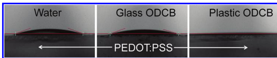
Figure 3. Image of contact angle measurement for water, glass-syringe handled ODCB, and plastic-syringe handled ODCB on PEDOT:PSS.
