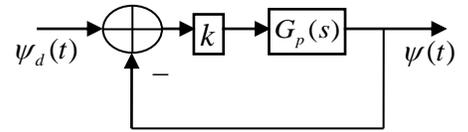
**Figure 2** Closed loop block diagram.
