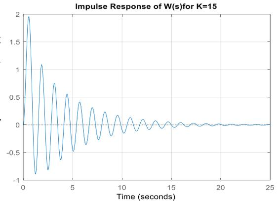
**Figure 3** Closed loop impulse response for  $K = 15$ .
