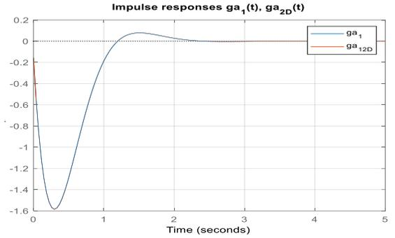
**Figure 2(d)** Impulse responses  $g_{\alpha_1}(t)$  and  $g_{\alpha_{2D}}(t)$ .
