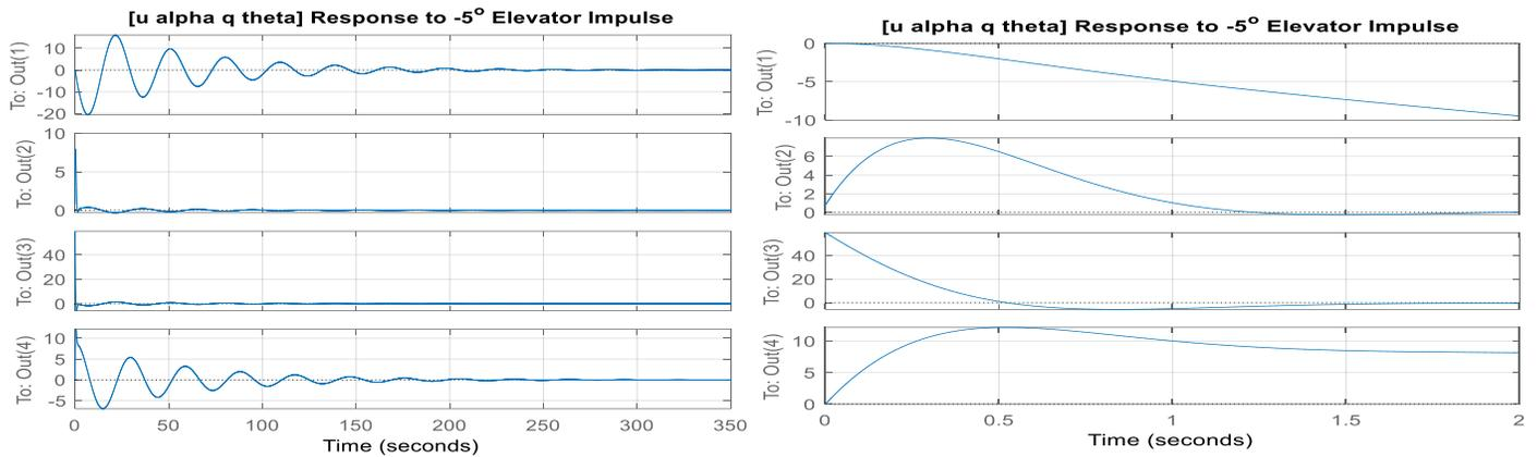
**Figure 1(d)** State response to  $\mathbf{u}(t) = -5^\circ \delta(t)$ : Complete response (LEFT), and initial response (RIGHT).
