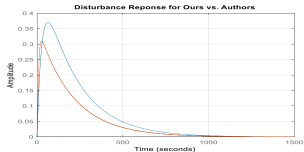
Figure 5. CL step responses for a unit step command (LEFT) and for a step disturbance T_d = 0.0175u(t) (RIGHT).
