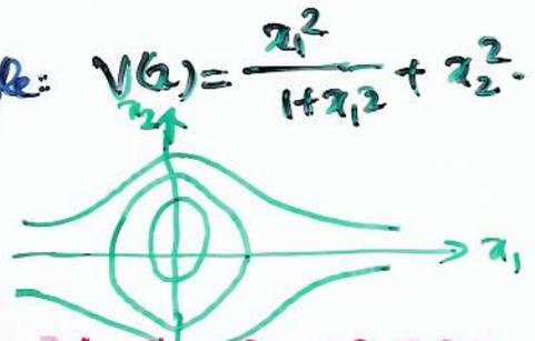
Work out:  $\min_{\|x\|=r} \left( \frac{x_1^2}{1+x_1^2} + x_2^2 \right) = \frac{r}{1+r} \xrightarrow{r \rightarrow \infty} 1 \Rightarrow \Omega_{\frac{1}{2}}$  is bounded.
