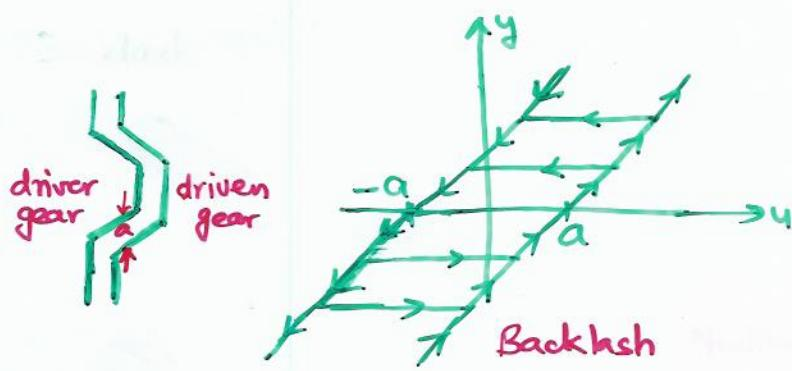
Backlash is seen between a pair of mating gears.
