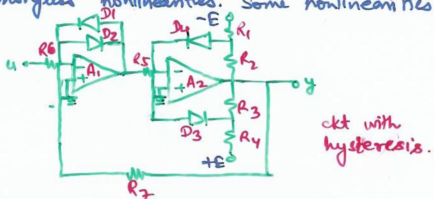
For low inputs, output is at  $L_-$ . Input increased to  $S_+$ , then output switches to  $L_+$  and stays there until input is decreased to  $S_-$ . (Example thermostat)
