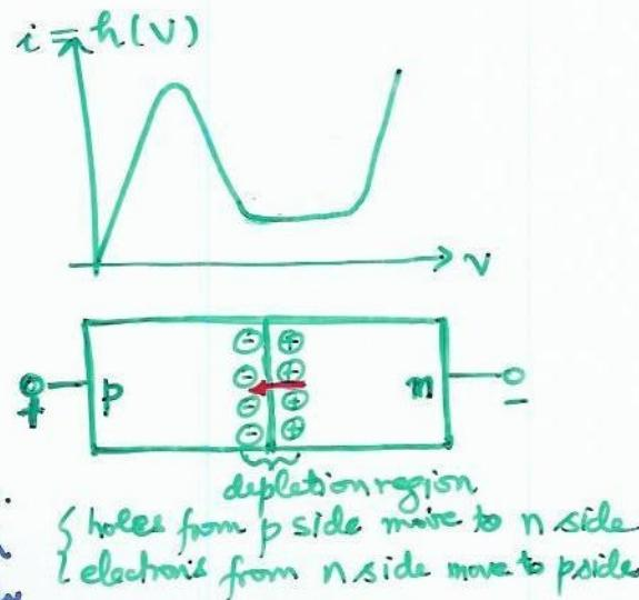
A -ve potential adds to this in-built electric field and so no current flows under "reverse bias". +ve potential has to first overcome this in-built electric field before current starts to flow in "forward bias".
