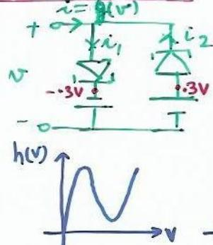
$$\begin{aligned} i &= i_1 - i_2 \\ &= h(v+3) - h(-3-v) \\ &= h(v+3) - h(-(v+3)) \end{aligned}$$
