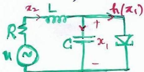
States: voltage across capacitor,  $z_1$ , current through inductor,  $z_2$
