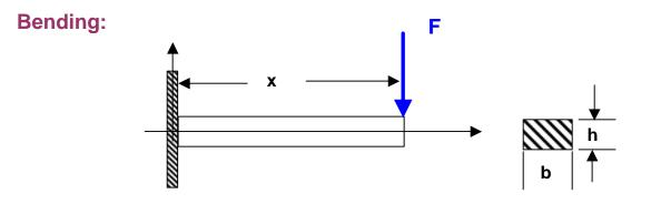
Bending is about z axis distance to neutral axis is (–y) Moment is F\*x
