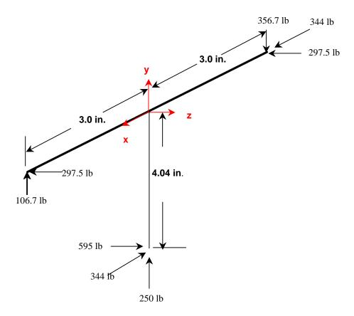
An engineer is required to specify bearings for the left and right ends of the 6.0" shaft.
