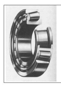
This bearing is called a **tapered roller bearing** it can handle radial loads as well as axial loads. Because of the taper on the rollers, radial loads will generate axial forces; tapered roller bearings are used in pair to counter the effect.
