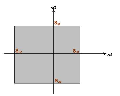
According to the **Maximum Normal Stress Theory**, if the principal stresses fall in this box, the part will not fail.
