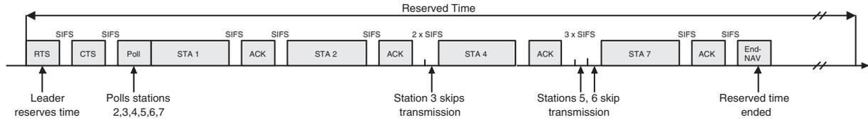
**Figure 4.** The group leader (station 1) reserves transmission time for its group and polls stations 2, 3, 4, 5, 6, 7. Stations 3, 5, 6 don't have packets. The reserved time is ended with an *End-NAV* packet by the leader.
