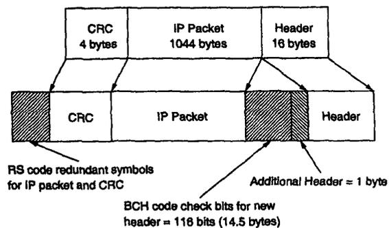
Fig. 5. Modified WaveLAN MAC frame structure
