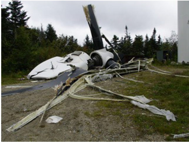
Fig. 4. Wind turbine failure from high winds shortly after a blade was repaired. Photo by Green Mountain Power, NREL 16713.
