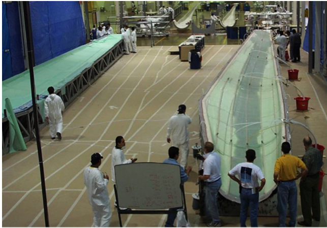
Fig. 11. Manufacturing of a wind turbine blade. Two outer shell halves can be seen. Photo from SNL.
