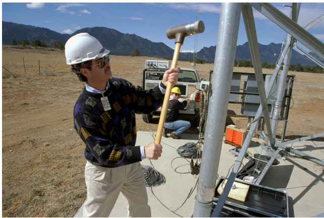
Fig. 5. Dynamic characterization testing of a turbine in 1999. The tower is struck with a hammer and the resulting vibrations are measured with accelerometers. Photo by David Parsons, NREL 07388.
