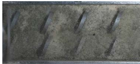
Dual co-currently rotating screws mix and convey heat carrier and biomass
