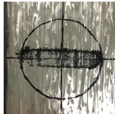
Figure 2: No Magnet Wear Debris Pattern
