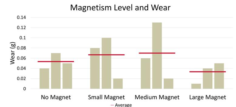
Figure 8: Magnetism Level and Corresponding Wear Data
