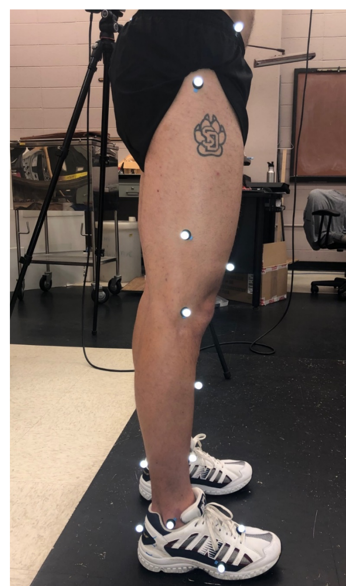
Figure 2: Reflective markers placement for motion tracking
