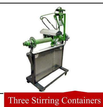
Figure 3: Experimental Stirring Container **Figure 4: Control Container** Six containers, three equipped with vertical stirring augers (Fig. 3) and three without (Fig. 4), were used to contain the wheat. The containers and stirrers that were designed and built by Sukup Manufacturing Company based on their Fastir stirring machine product.
