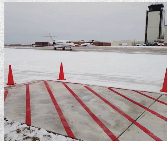
Halil Ceylan's research team has built the world's first electrically conductive heated pavement test site at an airport. This photo shows the technology performing well during a snow event on Dec. 10, 2016, at the Des Moines International Airport.
