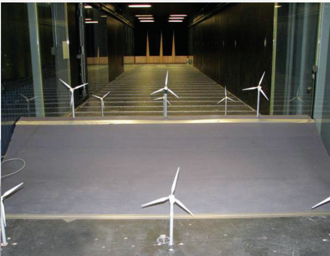
Wind turbines in the aeronautic and atmospheric boundary layer wind tunnel aligned to simulate a wind farm in complex terrain.
