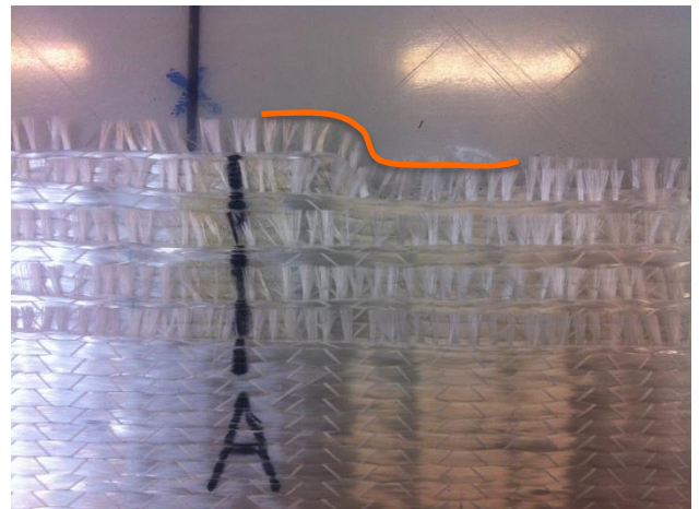
Figure 33: Outline of Ply 1. In-plane deformation after smoothing out by rolling
