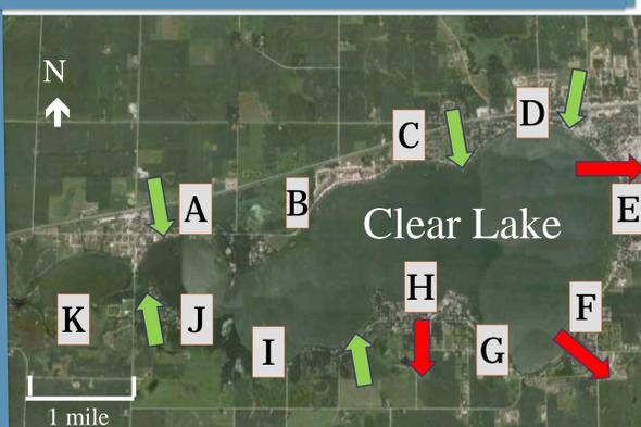
**Figure 1:** Monitoring well nest locations. Arrows indicate groundwater flow direction.
